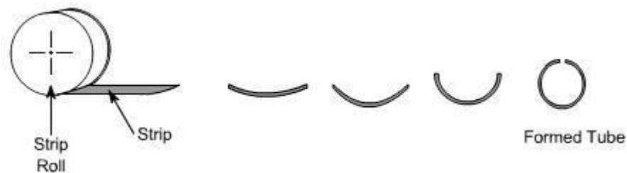
Fig 11.10: Forming of Tube from Strip
